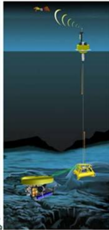
UTROV performs a task on an instrumented mooring, with communications over distances of less than 100 meters via an optical modem and then via electrical cable and satellite to shore-based operators.
