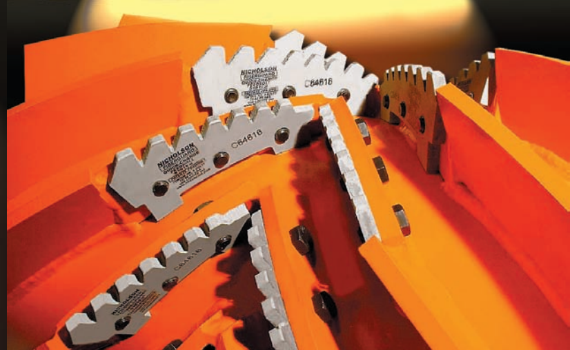
TYPE 'D' FIBERGUARD FEEDROLL INSERTS AFTER 7.5 MONTHS OF 2 AND 3 SHIFT HARDWOOD SAWMILL OPERATION: NICHOLSON 27 INCH DEBARKER.
