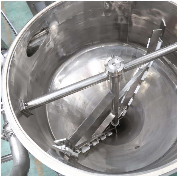
Inside Anchor Mixer of PVC-500 Mixer
